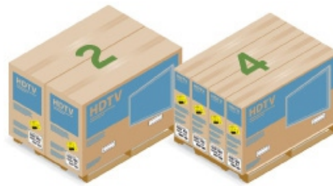
Using conventional cushioning foam (left), a large flat-screen television with its stand can be packed with only two units to a standard pallet. Switching to ARCEL resin (right) and removing the stand allows for cartons approximately half the size, easily doubling the yield.
